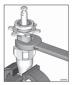
11. Install o-ring onto packing nut. Torque to 75  $\pm$  5 in-lb (8.5  $\pm$  0.5 N•m) or additional 1/2 turn from hand tight.
