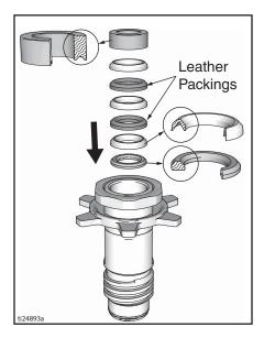
5. Loosely install packing nut with o-ring onto cylinder.
