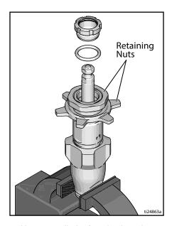
2. Unscrew cylinder from intake valve.
