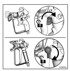
7. Hold a metal part of the gun firmly to a grounded metal pail. Trigger the gun to relieve pressure.
