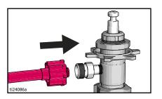
Move pump displacement rod up or down until it slides into the connecting rod when the pump is slid into the drive housing.
