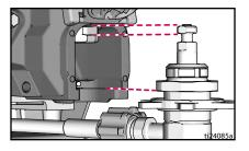
Slide pump all the way into drive housing.
