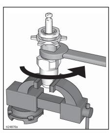
Dissemble intake valve. Clean and inspect. O-ring may require a pick for removal.
