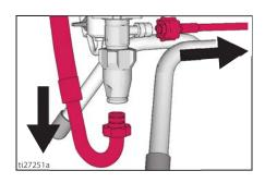
5. Slide pump out of the drive housing.
