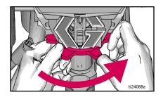
Use a hammer to turn pump retaining nut an additional 1/8 to 1/6th turn or 45° to 60°.
