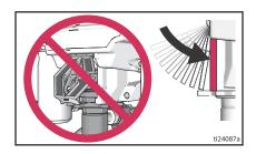
Use both hands to tighten pump retaining nut.
