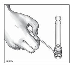
Grease top inch or two of piston rod that will go through the cylinder throat packings. Gently guide displacement rod up through throat packings. Tap bottom of piston valve as necessary with a leather or plastic hammer.
